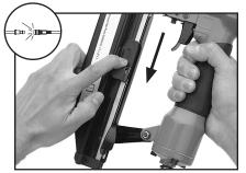
Figure 5. Sliding magazine pusher back.
